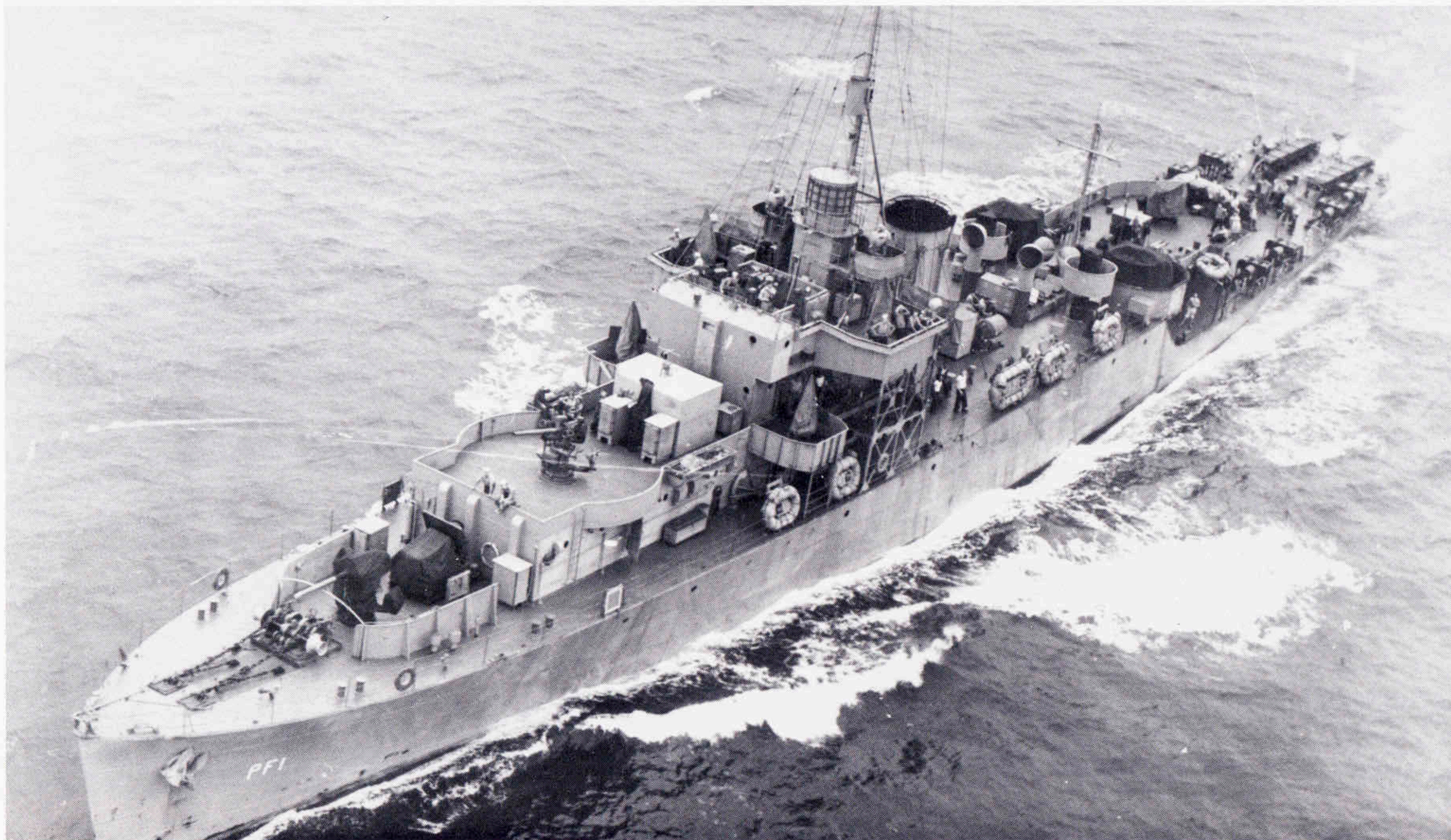
The Second USS Asheville Ship Identification: PF-1 Displacement: 1,335 tons Length: 301' 6" Beam: 36' 6" Draft: 13' 8" Speed: 20 knots Crew: 194 Weapons: Three three inch guns Commissioned: December 1, 1942 Decommissioned: January 14, 1946.
